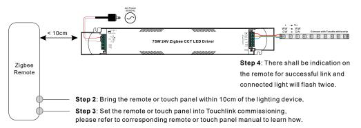
Note: 1) Directly TouchLink (both not added to a ZigBee network), each device can link with 1 remote.
